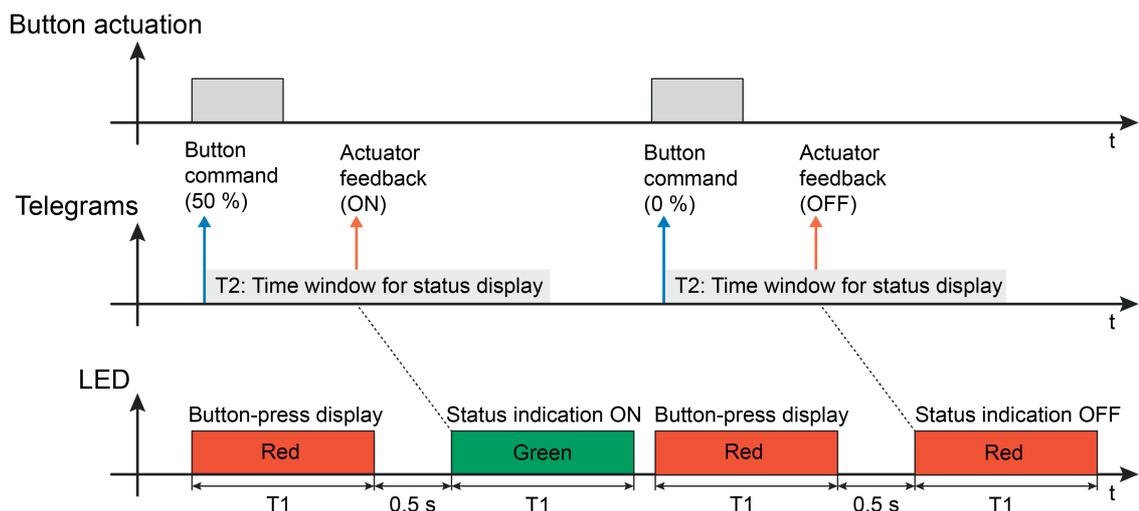
Figure 20: Example of a status display with the operating function "Value transmitter 1-byte" with double status (ON and OFF) Telegram on pressing the button
