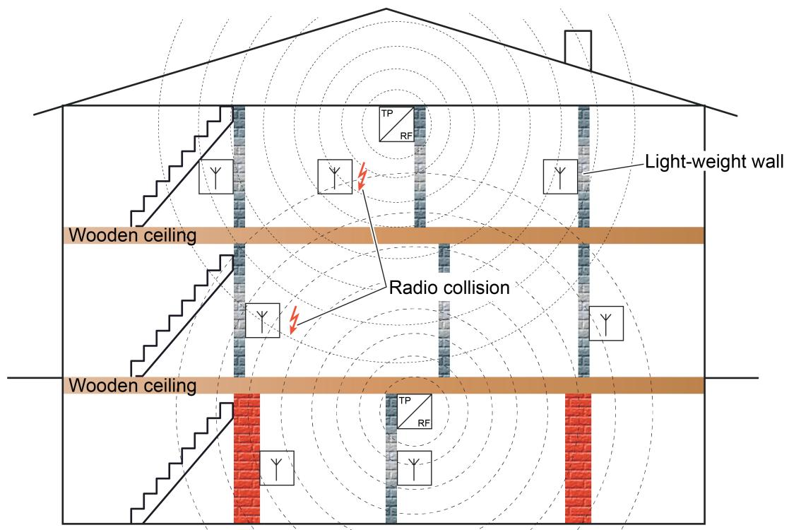
Figure 35: Building structure with two KNX RF lines, disadvantageous influence (example)
