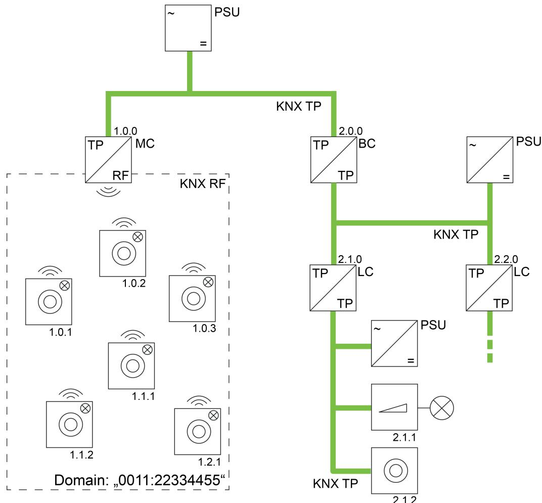
Figure 40: Example of a possible KNX topology with RF and TP lines
