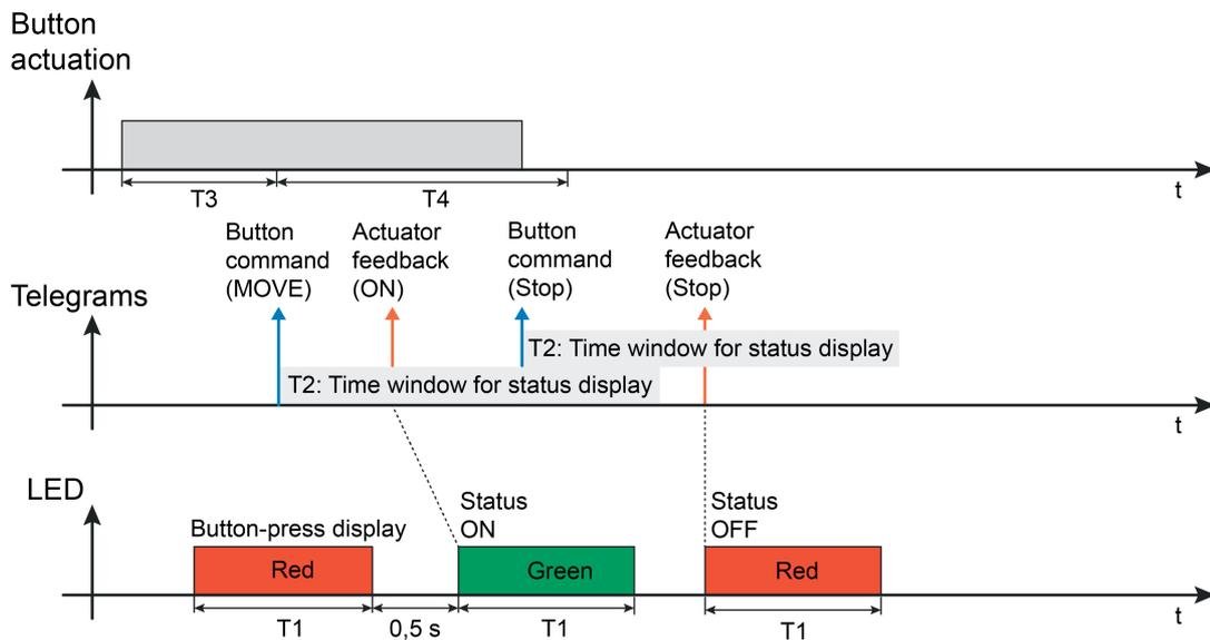
Figure 19: Example of a status display with the operating function "Venetian blind" with a long button-press
