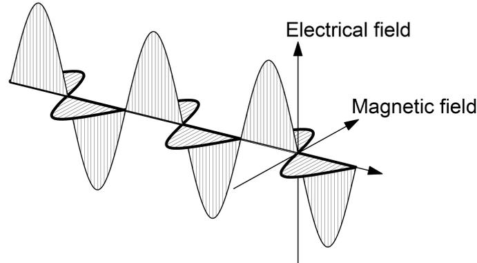
Figure 25: Model of an electromagnetic wave in an open space
