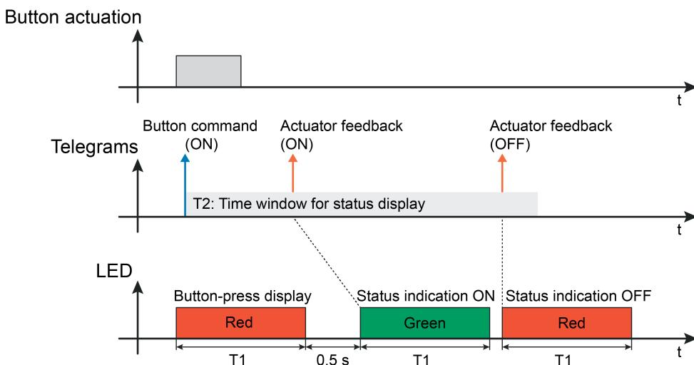
Figure 9: Example of a two-level actuation and status display with double status
