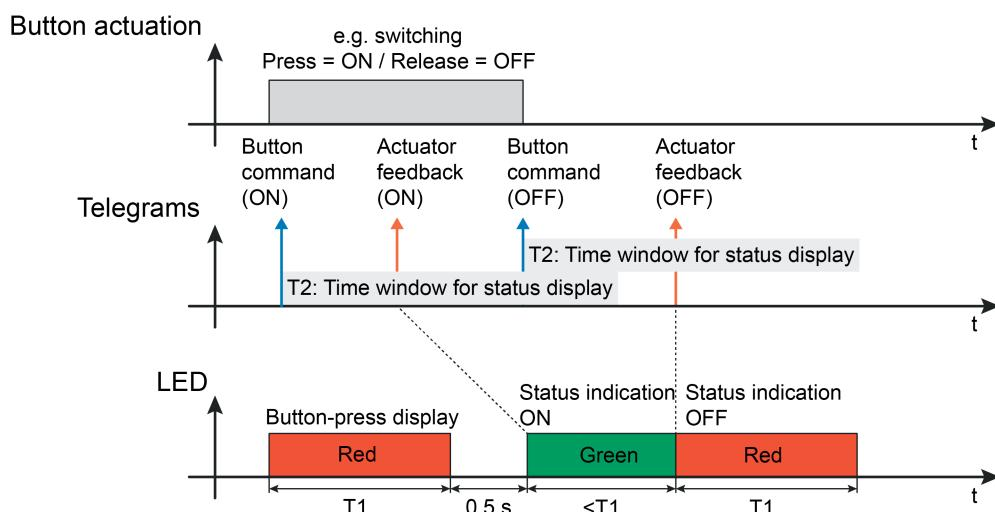
Figure 8: Example of a two-level actuation and status display with double status
