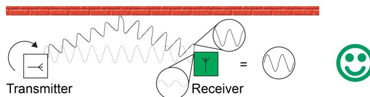
Figure 33: Reflection allows reception through a change of polarisation
