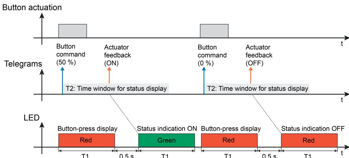
Figure 20: Example of a status display with the operating function "Value transmitter 1-byte" with double status (ON and OFF)
