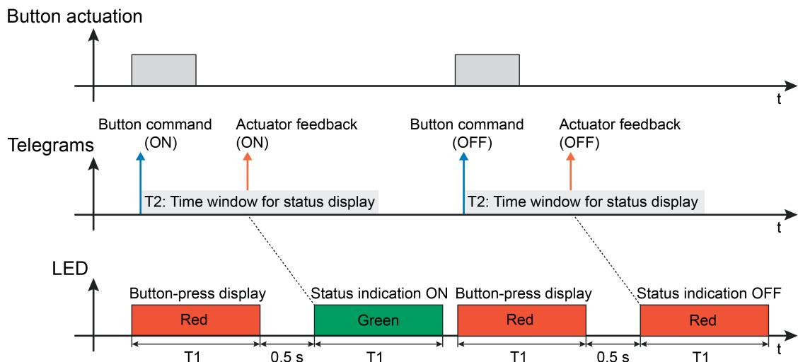
Figure 13: Example of a status display with the operating function "Switching" with double status (ON and OFF)
