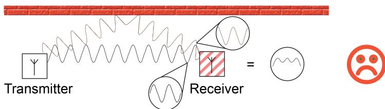
Figure 32: Interference at the receiver prevents reception
