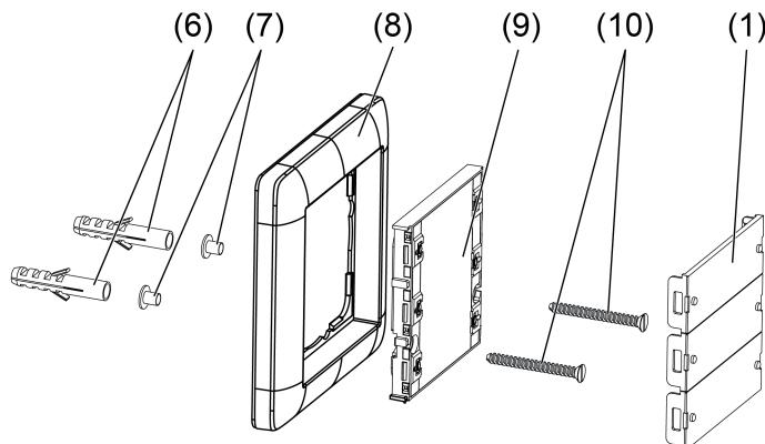
Figure 2: Screw mounting
