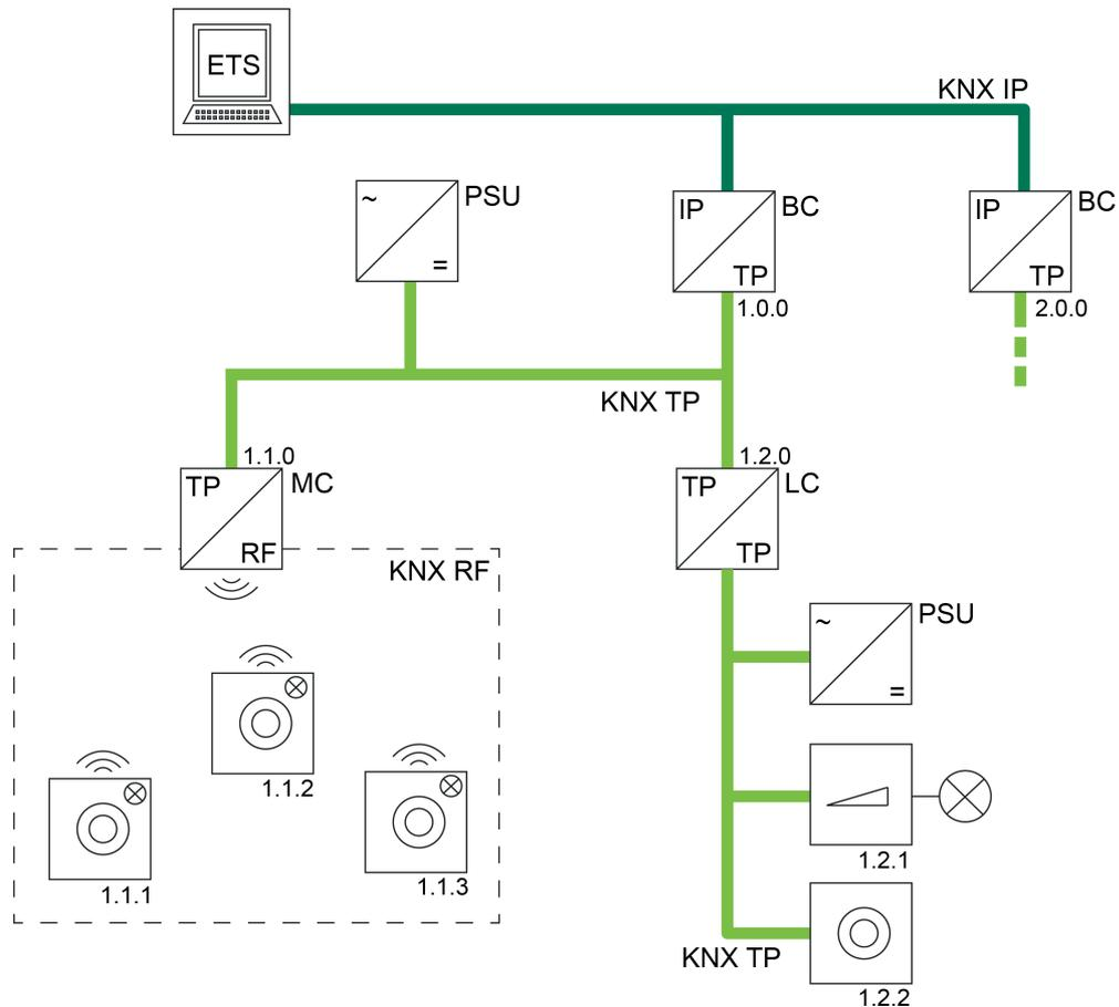
Figure 44: Example of a possible KNX topology with one KNX IP connection of the ETS (KNX/net IP)
