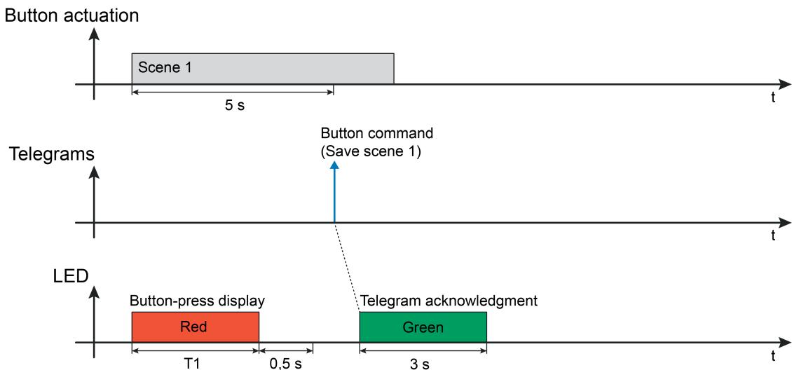
Figure 23: Example of an LED display with the operating function "Scene extension"
