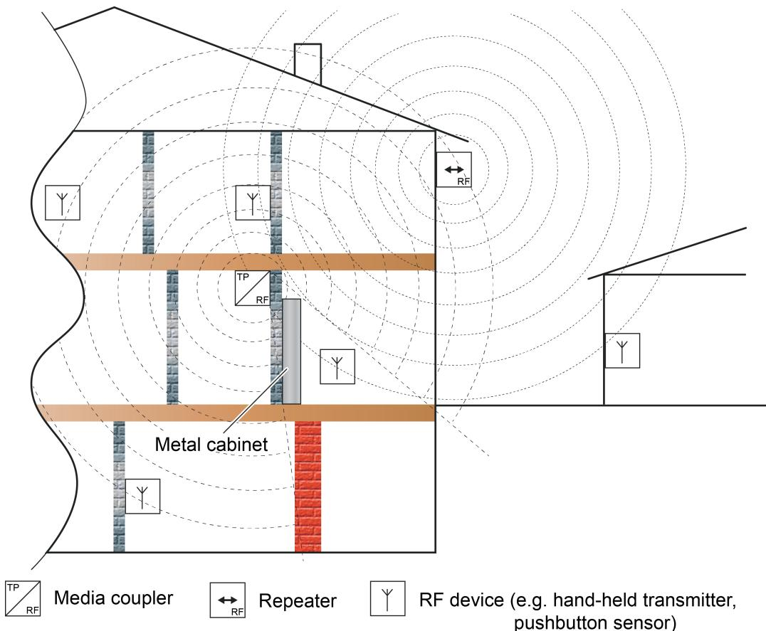
Figure 38: Use of a media coupler as a repeater for signal amplification and elimination of radio shadow for indoor and outdoor applications
