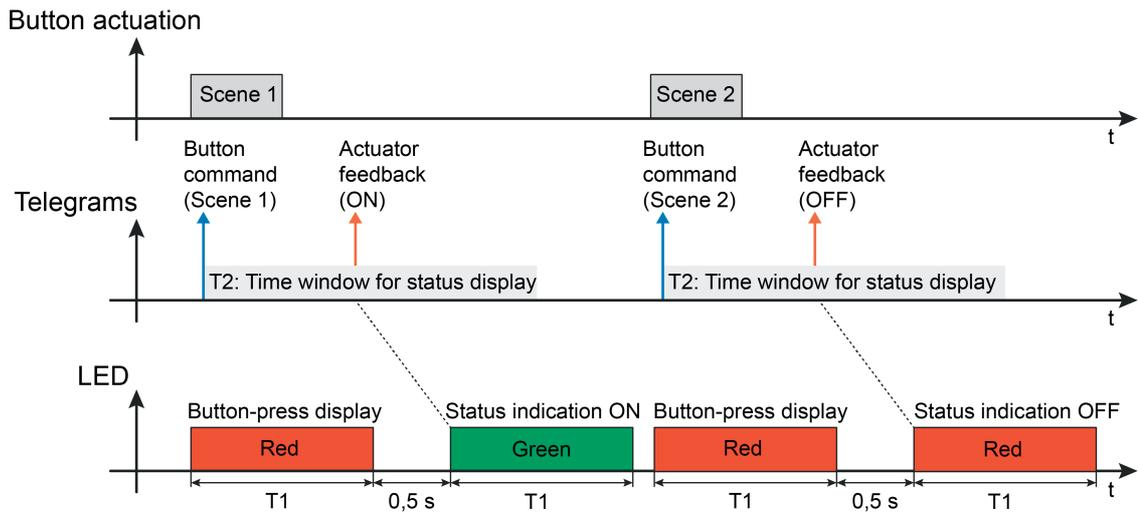
Figure 21: Example of a status display with the operating function "Scene extension"
