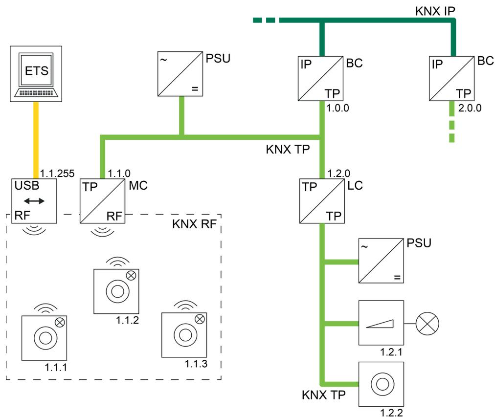
Figure 42: Example of a possible KNX topology with a KNX RF USB data interface
