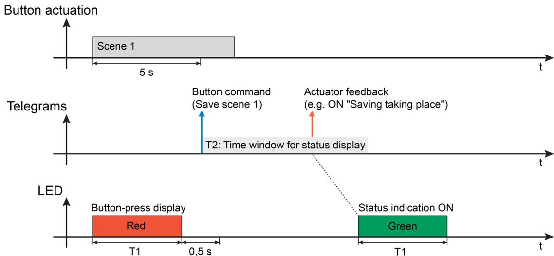
Figure 22: Example of a status display with the operating function "Scene extension"
