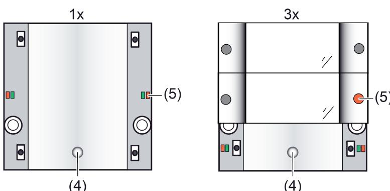
Figure 4: Programming button between the rocker cover (left: 1-gang / right: 3-gang)
