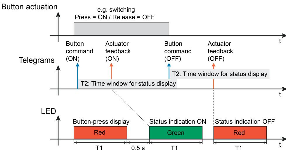
Figure 7: Example of a two-level actuation and status display with double status
