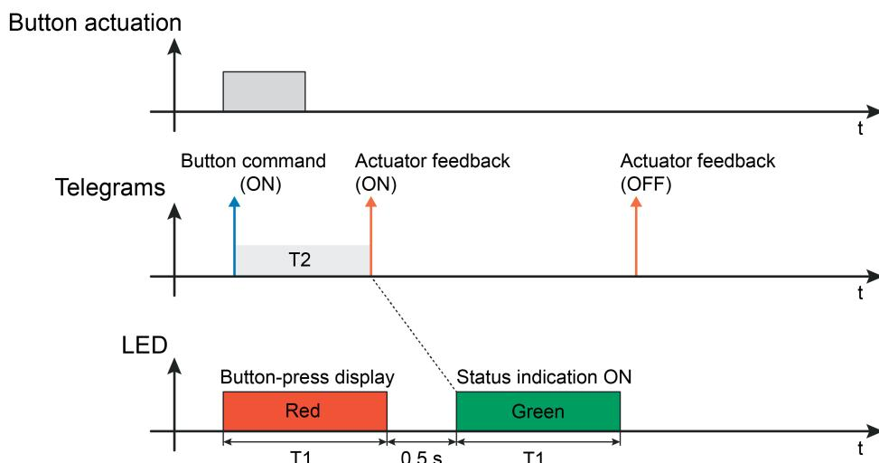
Figure 10: Example of a two-level actuation and status display with double status
