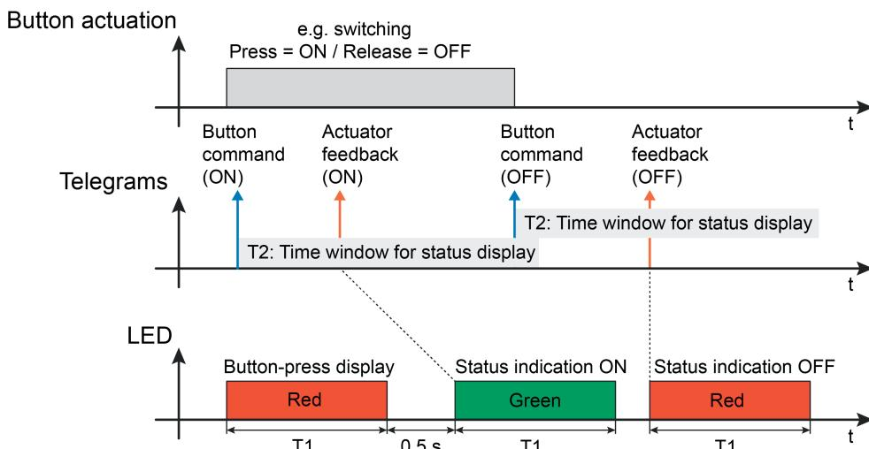
Figure 14: Example of a status display with the operating function "Switching" with double status (ON and OFF)
