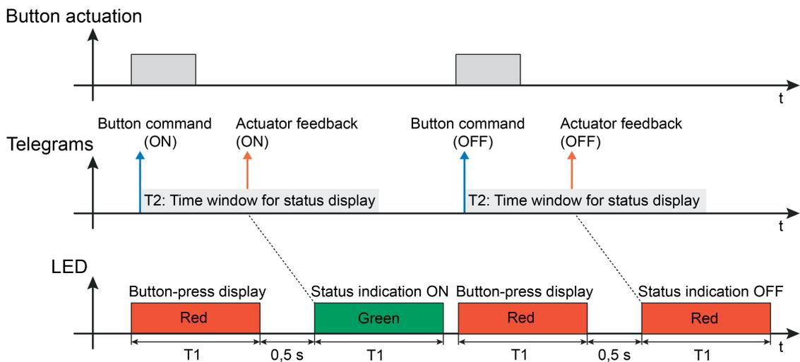
Figure 6: Example of a two-level actuation and status display with double status
