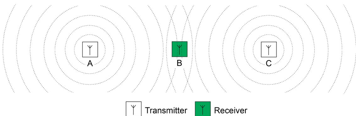
Figure 24: Radio collisions on the receiver due to the transmitter being too far away
