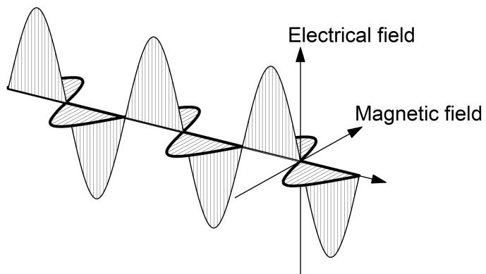
Figure 25: Model of an electromagnetic wave in an open space
