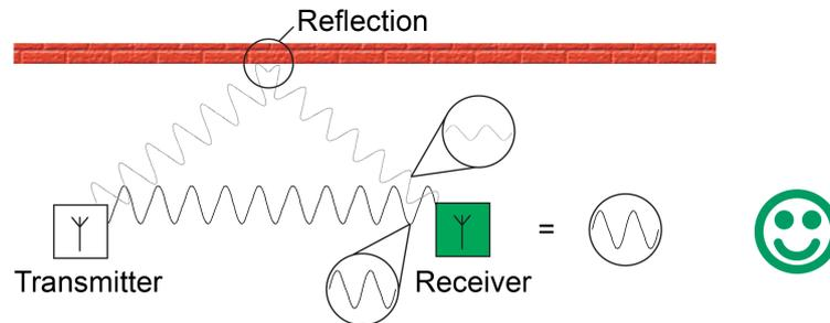
Figure 31: Interference has no effect on the receiver
