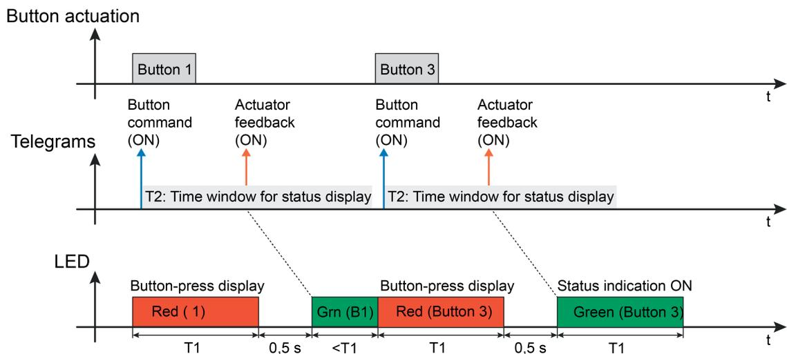
Figure 11: Example of a two-level actuation and status display
