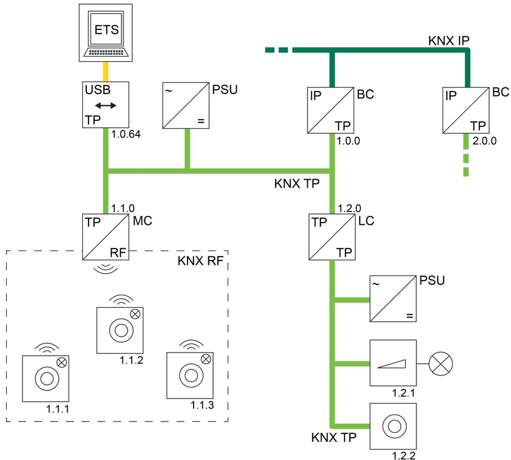
Figure 43: Example of a possible KNX topology with a KNX TP USB data interface
