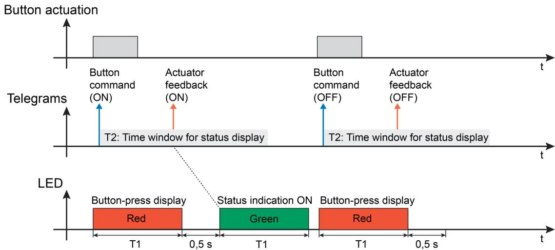
Figure 5: Example of a two-level actuation and status display with single status
