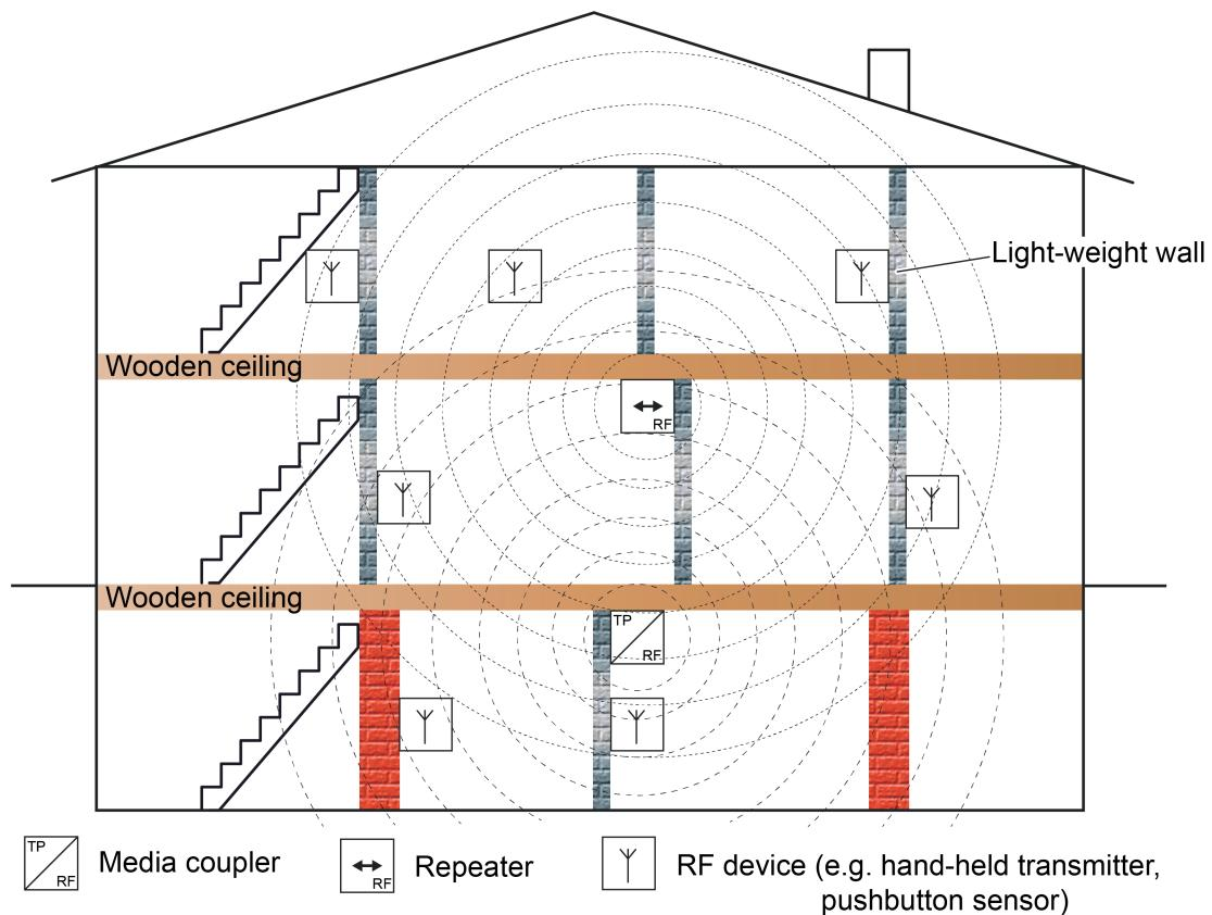
Figure 36: Building structure with one KNX RF line and repeater (example)
