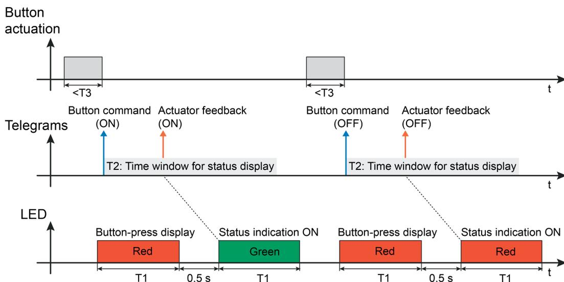
Figure 15: Example of a status display with the operating function "Dimming" with a short button-press (with double status ON and OFF)
