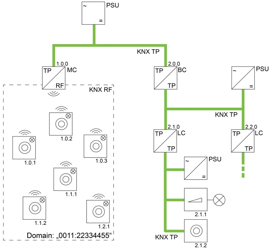
Figure 40: Example of a possible KNX topology with RF and TP lines
