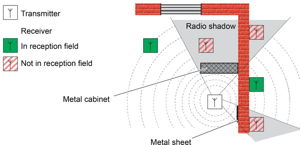
Figure 30: Radio shadow in a building due to metallic parts (idealised)
