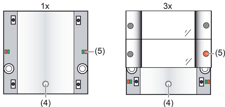
Figure 4: Programming button between the rocker cover (left: 1-gang / right: 3-gang)
