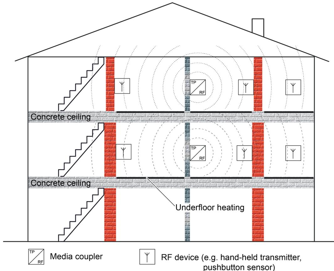
Figure 37: Building structure with two KNX RF lines, which do not influence each other negatively due to the building consistency (example)
