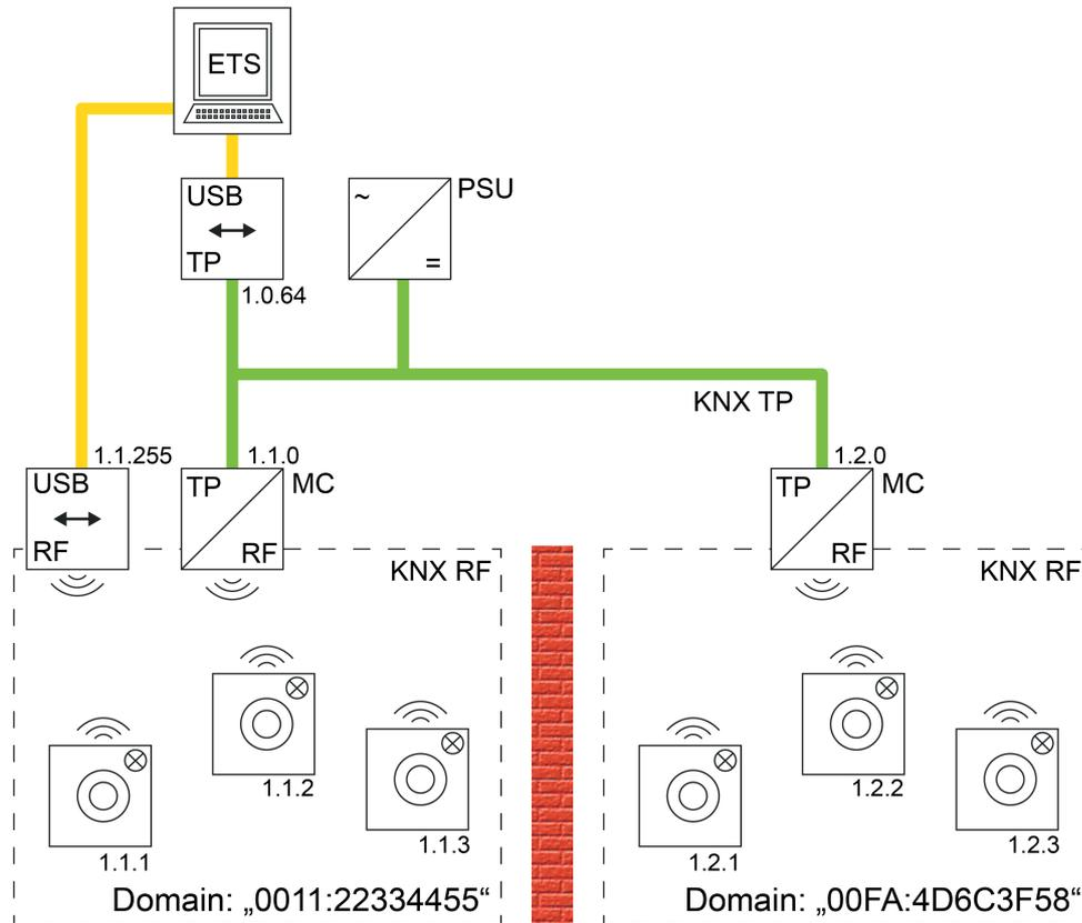
Figure 41: Example of a possible KNX topology with two RF lines and coupling via a TP main line (example)
