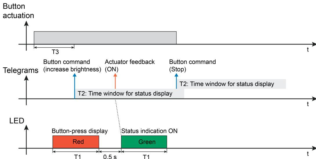
Figure 16: Example of a status display with the operating function "Dimming" with a long button-press
