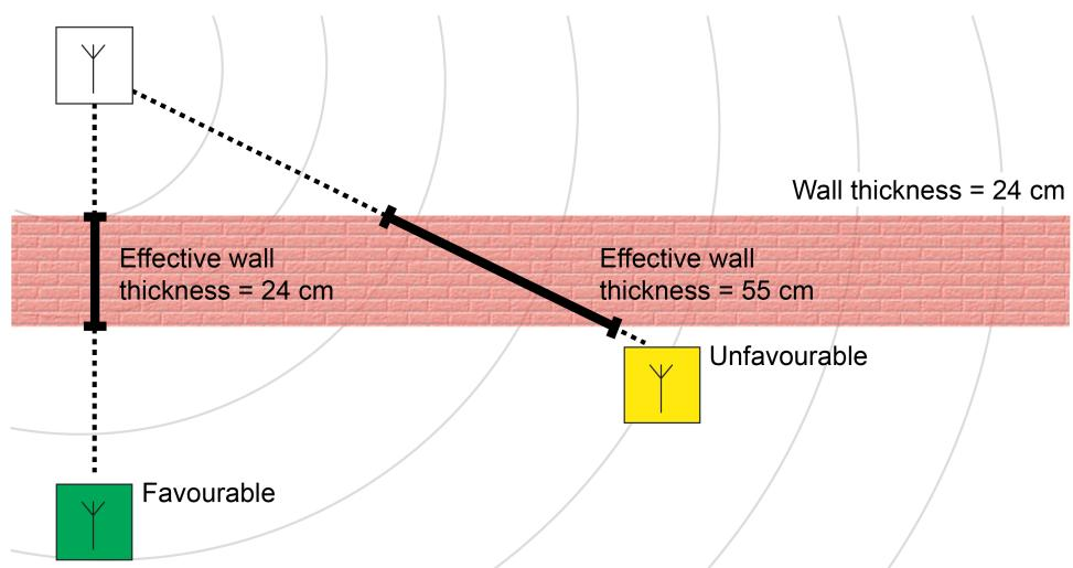
Figure 29: Attenuation through effective wall or ceiling thickness
