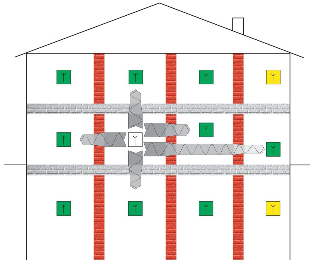
Figure 28: Attenuation of the radio signal in buildings through walls and ceilings
