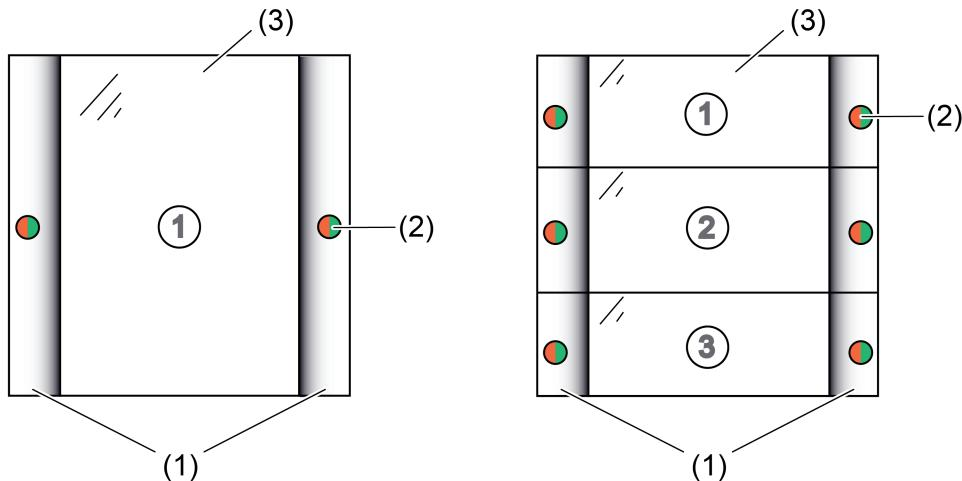
Figure 1: Device components Push-button sensor, 1-gang (left) and 3-gang (right)
