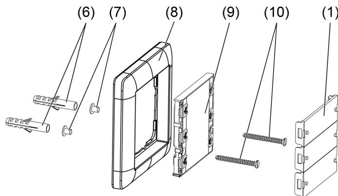
Figure 2: Screw mounting
