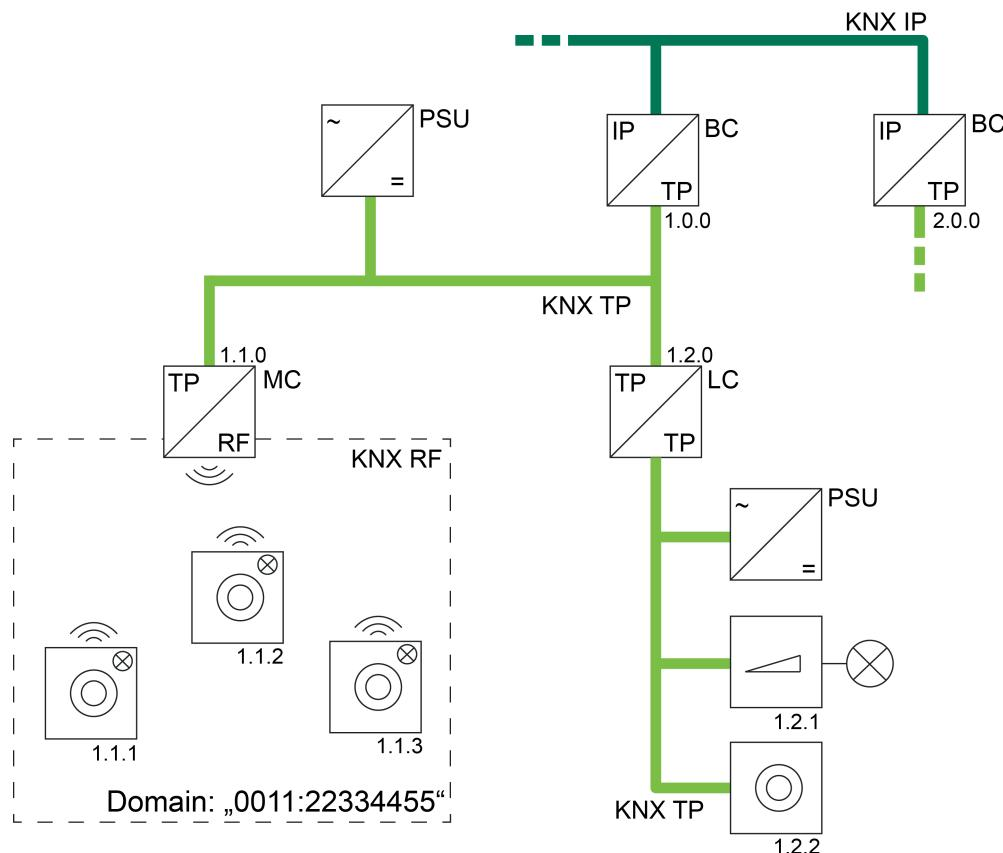
Figure 39: Example of a possible KNX topology with RF, TP and IP lines
