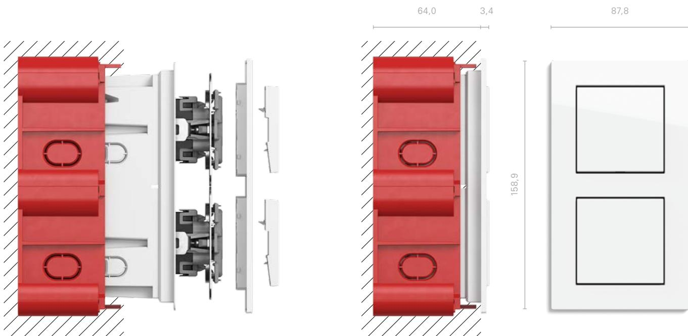
Installation in cavity walls
