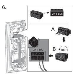
Trim connection cable to length and connect to plug terminal (A). Rotate plug terminal by 180° (B) and attach to the connector of the voice module or door station module.
