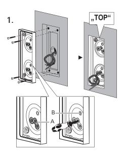
Select an opening (A) for the cable feed-through and pierce it with a round object (no cross-shaped cut).
