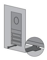
Gently tighten the screw to lock the housing using the enclosed locking key (0,6 Nm). The application angle is 90°.
