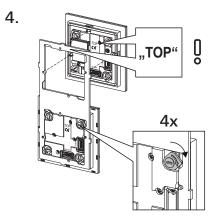
Insert the modules into the function carrier (observe TOP marking) and lock (slot screwdriver  $4 \times 0.8$  mm). For detailed information on the module please refer to the operating instructions of the individual modules.
