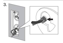
Strip insulation of the connection cable as close as possible to the seal cap (see arrow). The stripped part of the connection cable may not be behind the seal cap as this does not guarantee a functional seal.
