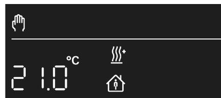
Figure 3: Setpoint temperature display in manual mode
