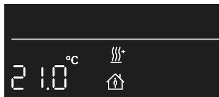
Figure 2: Setpoint temperature display in automatic mode
