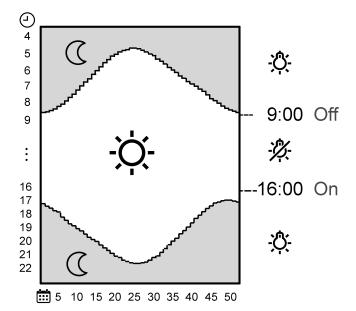
Figure 6: Default setting: Astro function for switching and dimming inserts
