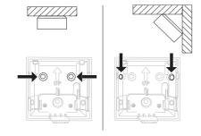
Install the mounting frame on the wall. The disconnecting surface of the tamper contact (see arrow) must be secured with a screw.
