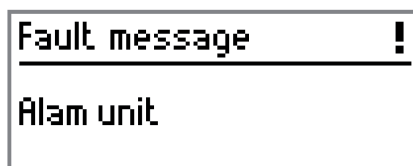
Figure 65: Example of a one-line fault message display
