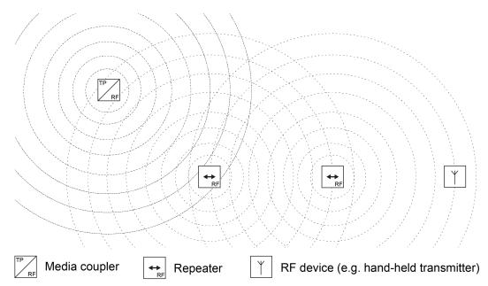
Image 8: Application example 2: two repeaters in a strand configuration
