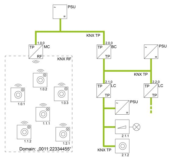
Image 2: Example of a possible KNX topology with RF and TP lines Media coupler as backbone coupler
