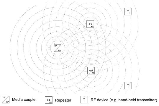
Image 7: Application example 1: two repeaters in a star configuration
