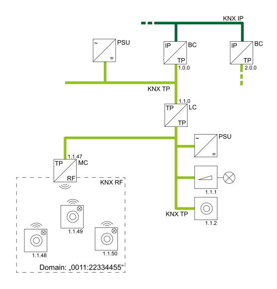
Image 4: Example of a possible KNX topology with RF and TP segments
