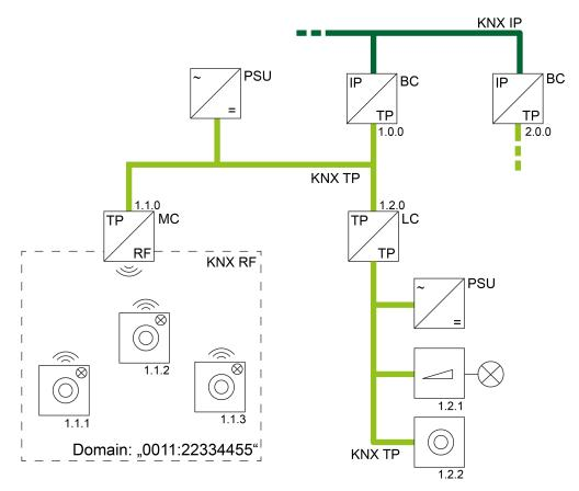
Image 3: Example of a possible KNX topology with RF, TP and IP lines
