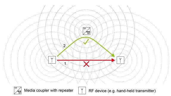
Image 6: Application example of a media coupler with repeater function
