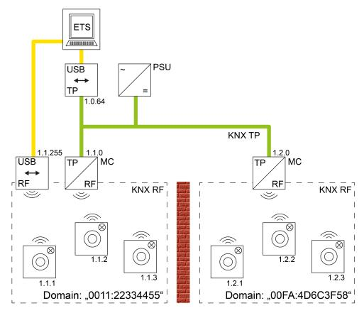
Image 5: Example of a possible KNX topology with two RF lines and coupling via a main TP line
