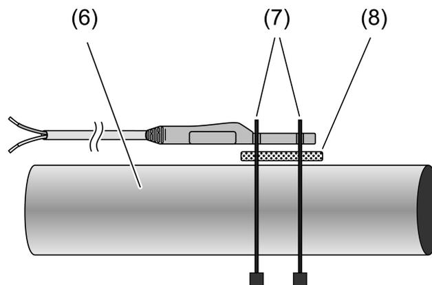
Figure 2: Fitting to a pipe with cable ties
