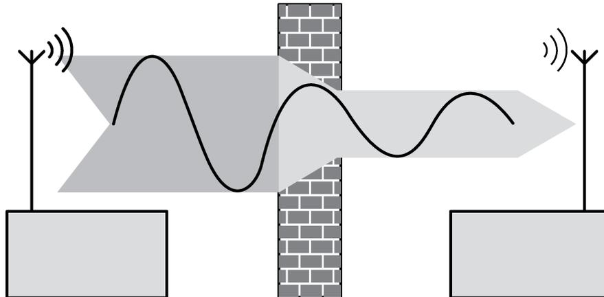
Figure 2: Reduced range due to structural obstacles
