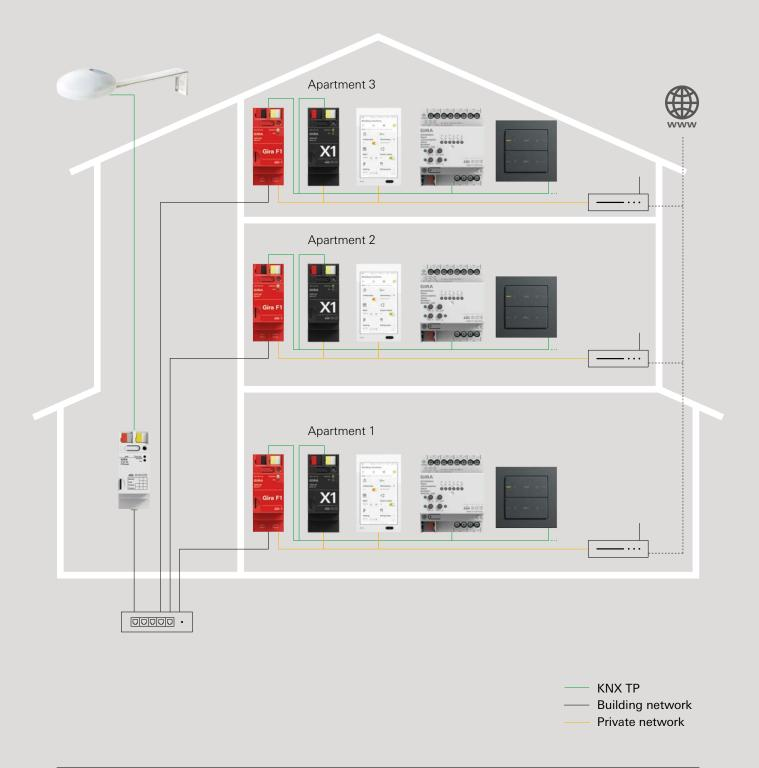
The Gira F1 firewall module is installed in the control cabinet as part of a KNX system. Following start-up, the Gira F1 acts as a KNX bridge between several self-contained KNX systems.
