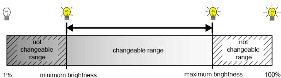
Figure 41: Brightness sequence during automatic brightness sequence
