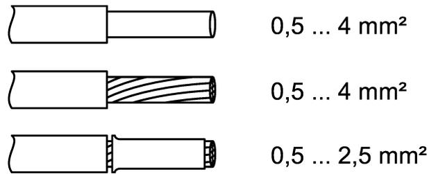
Figure 5: Clampable cable cross-sections
