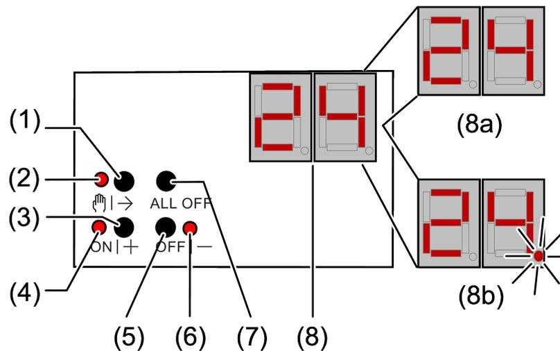
Figure 1: DALI Gateway control panel, 1fold
