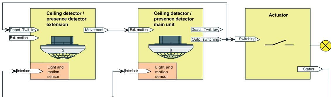
Figure 29: Application example with twilight level evaluation in the main unit and extensions for the data format "Switching"
