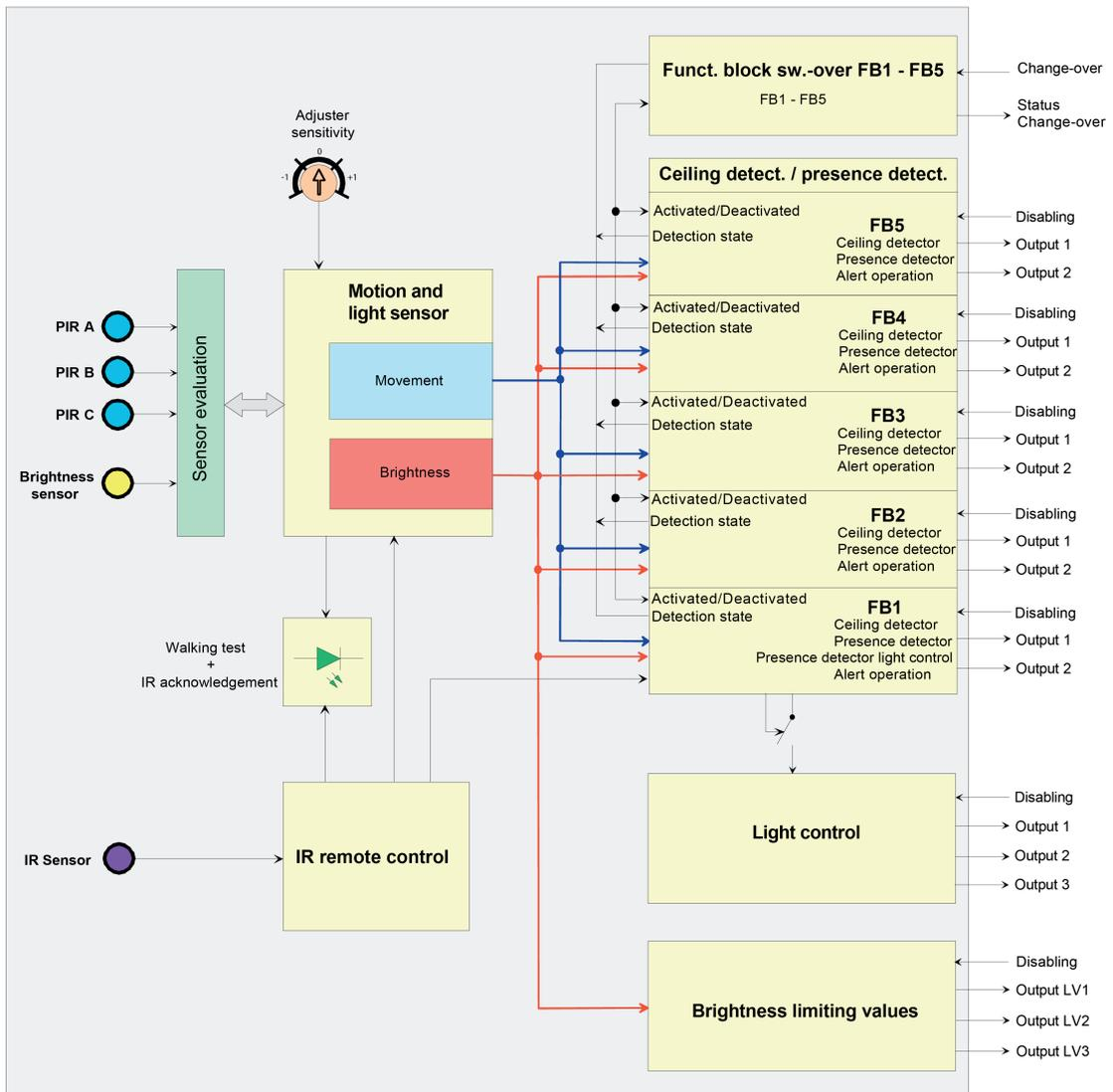
Figure 10: Block diagram of all device functions
