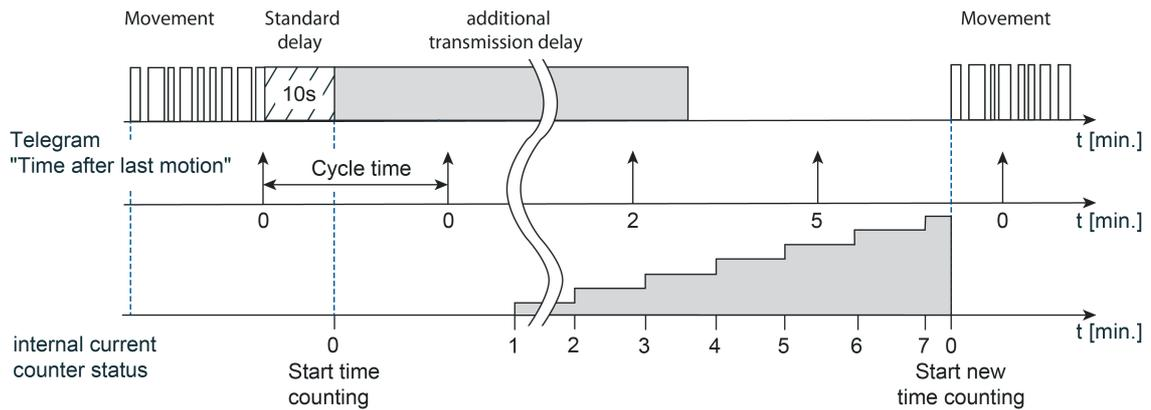
Figure 39: Measurement of the time period after last motion
