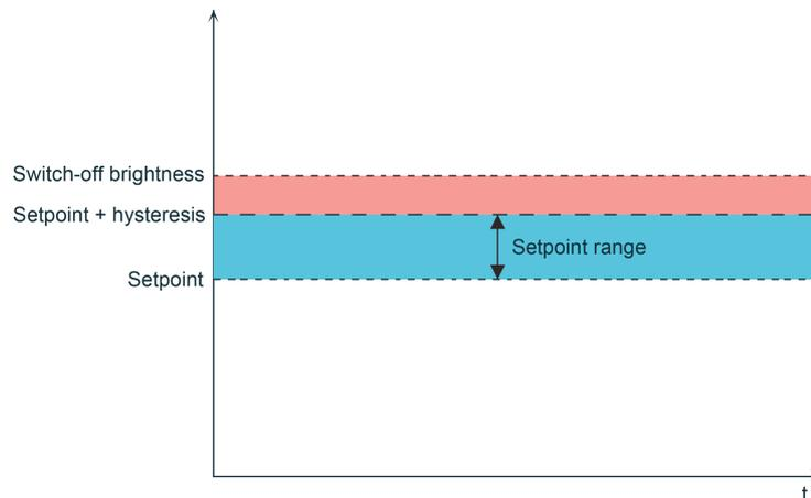
Figure 53: The switch-off brightness results relatively from the setpoint and hysteresis value of the setpoint
