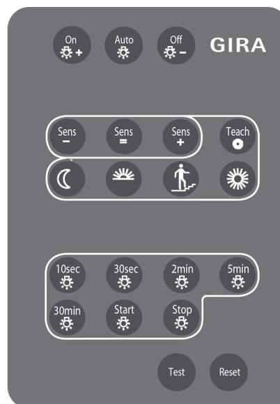
Figure 61: Buttons on the IR remote control
