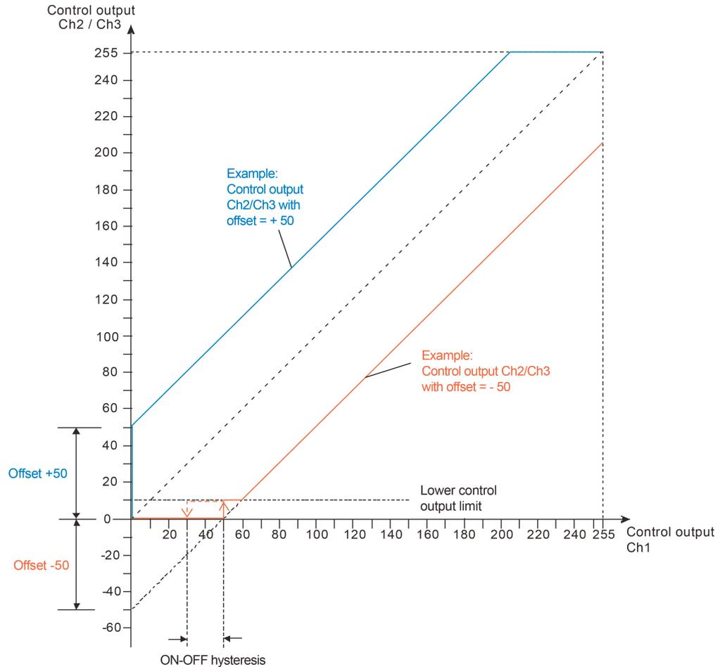
Figure 46: Control outputs of channels 2 or 3 dependent on the control output of channel 1
