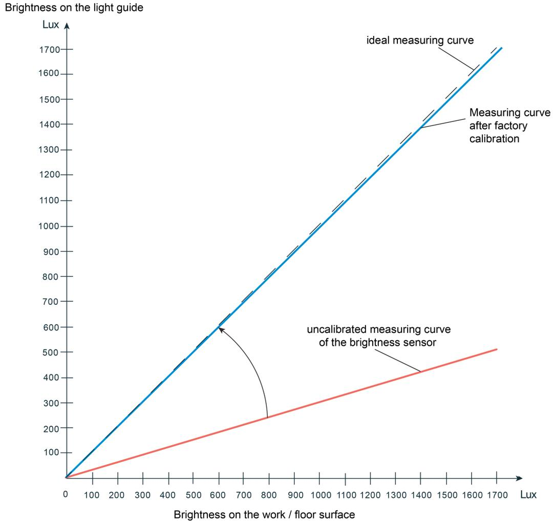
Figure 14: Determining the brightness on the work / floor surface during factory calibration
