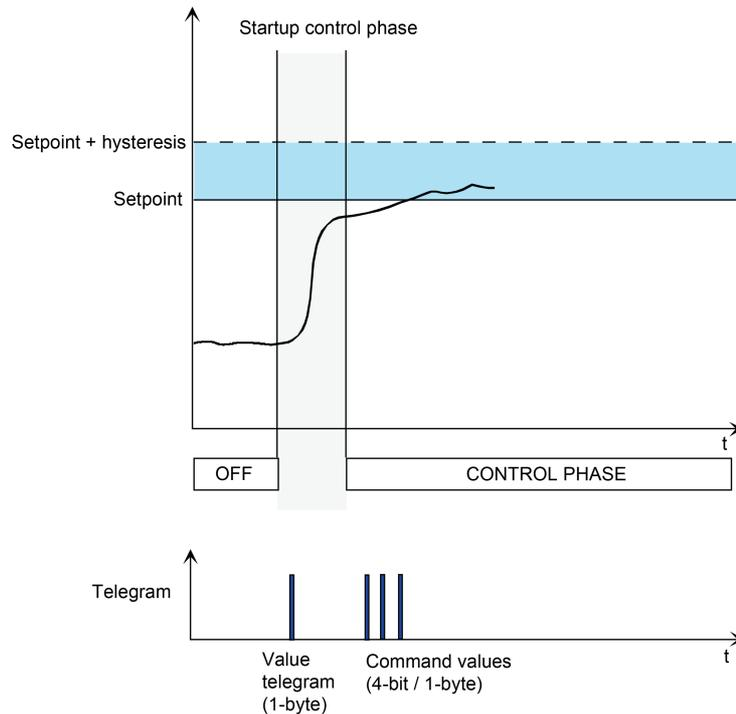
Figure 51: Startup control behaviour with absolute value telegrams (1-byte)
