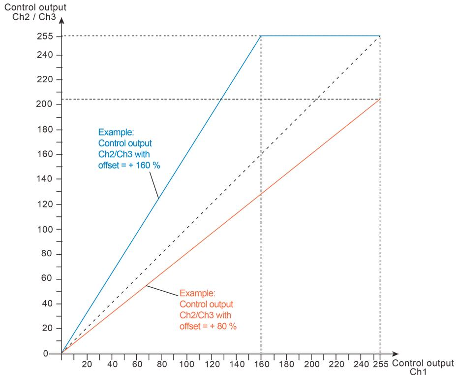
Figure 47: Control outputs of channels 2 or 3 dependent on the control output of channel 1
