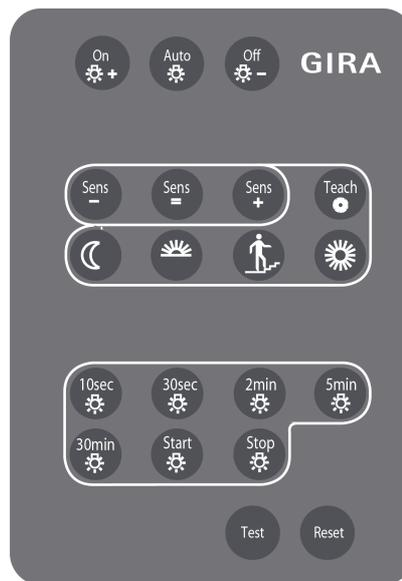
Figure 9: Buttons on the IR remote control
