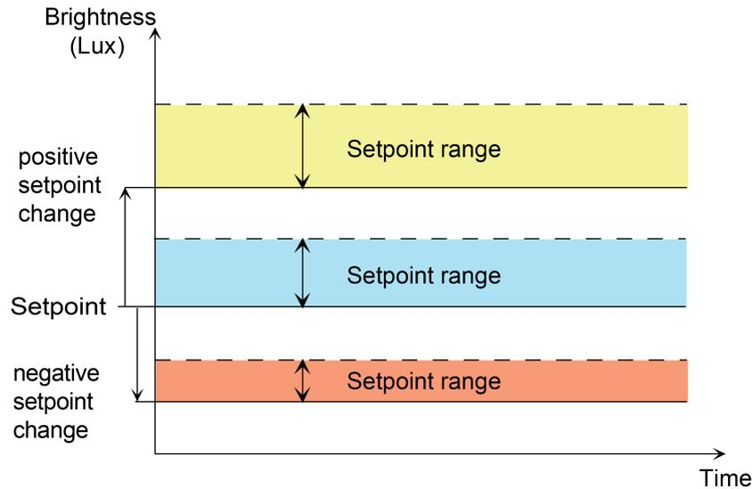
Figure 44: Shift of the setpoint range by means of setpoint adjustment
