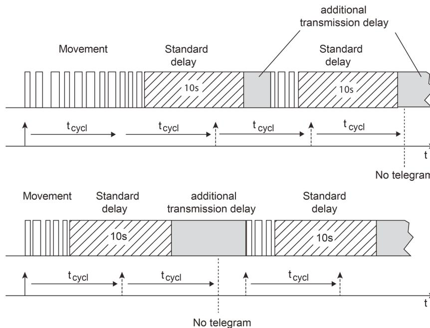
Figure 34: Cyclical transmission during a motion detection
