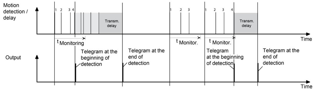
Figure 20: Motion evaluation with the detector
