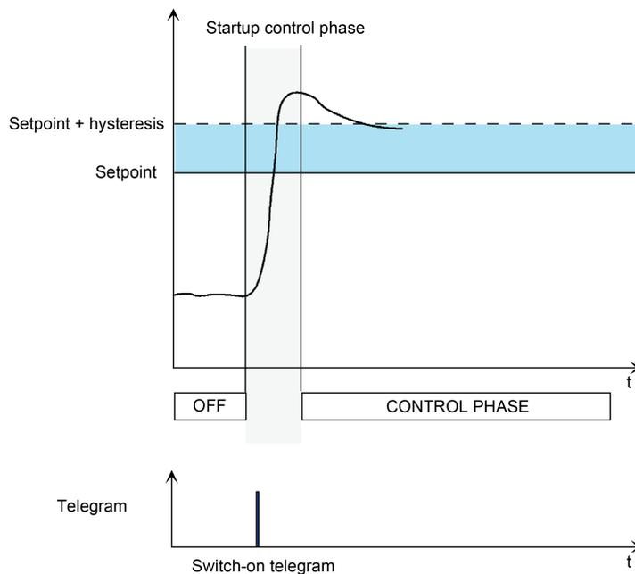
Figure 49: Startup control behaviour with switching telegram (1-bit)
