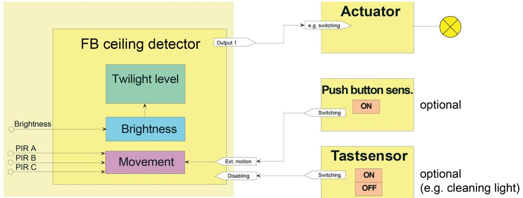
Figure 16: Application example of the application ceiling detector
