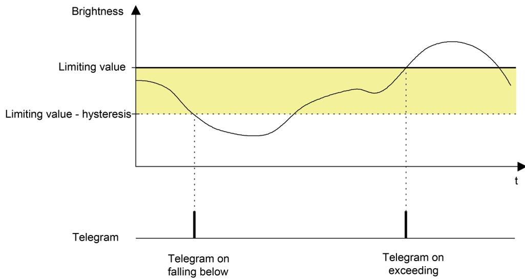
Figure 59: Example 1 of the limiting value definition
