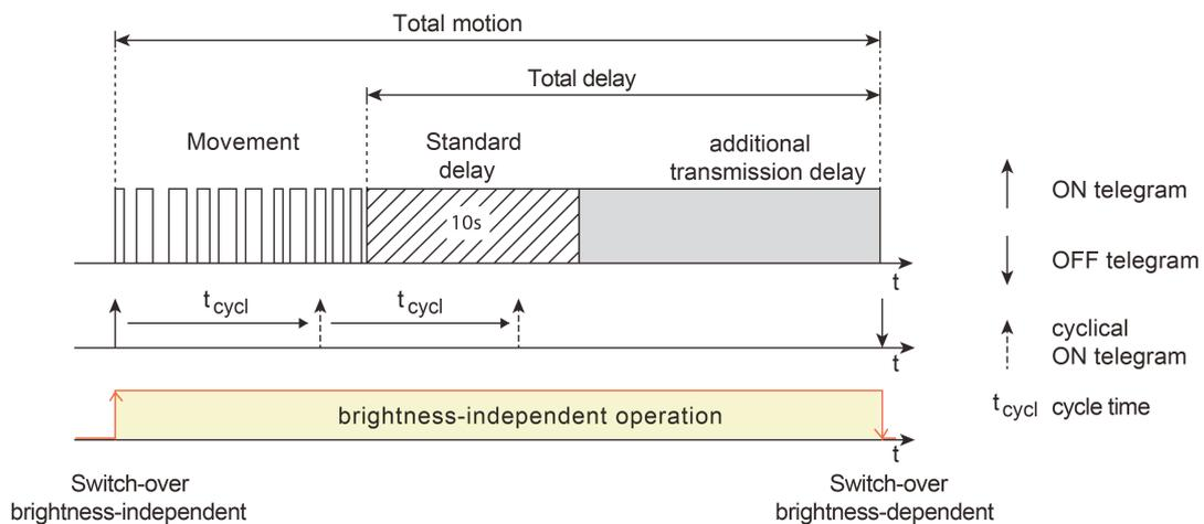
Figure 33: Total motion with motion detection, standard delay and additional transmission delay
