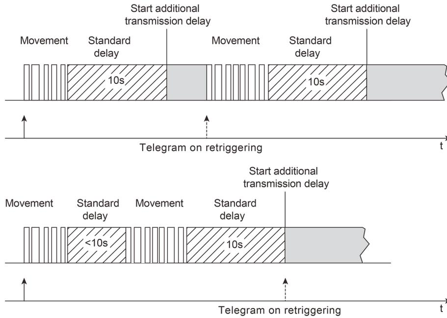
Figure 35: Triggering of a telegram when retriggering
