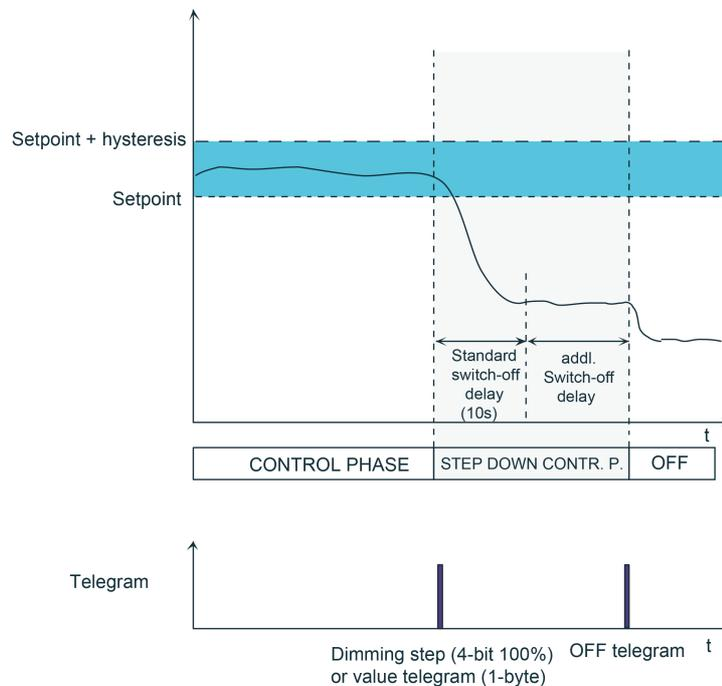
Figure 56: Step down control behaviour with waiting time
