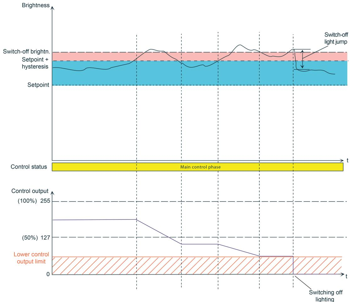
Figure 54: Example of a control output presetting with evaluation of the lower control output limit
