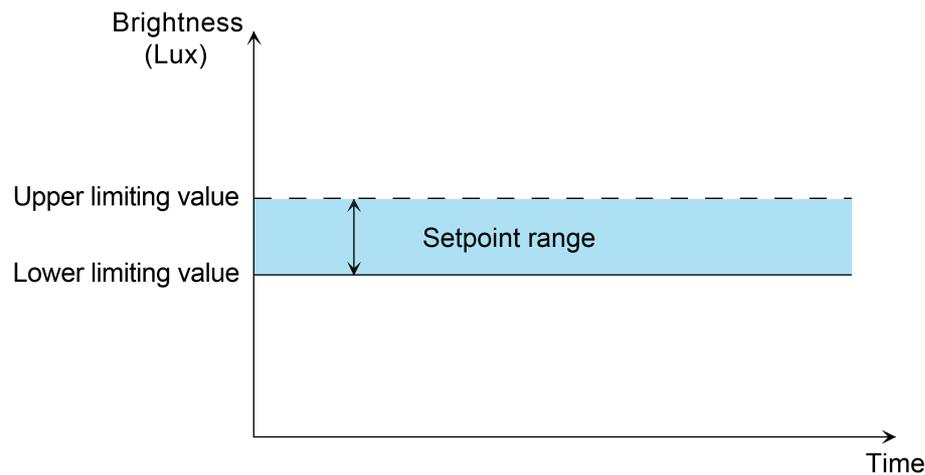
Figure 43: Setpoint range of the light control
