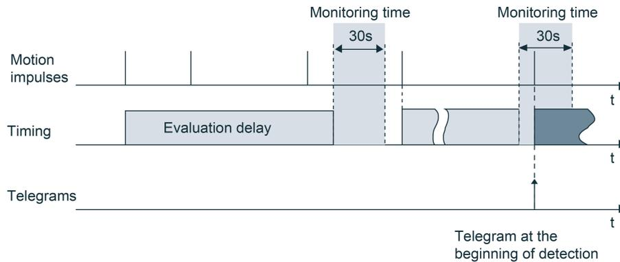
Figure 37: Evaluation delay with only brief motion
