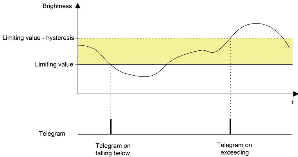
Figure 60: Example 2 of the limiting value definition
