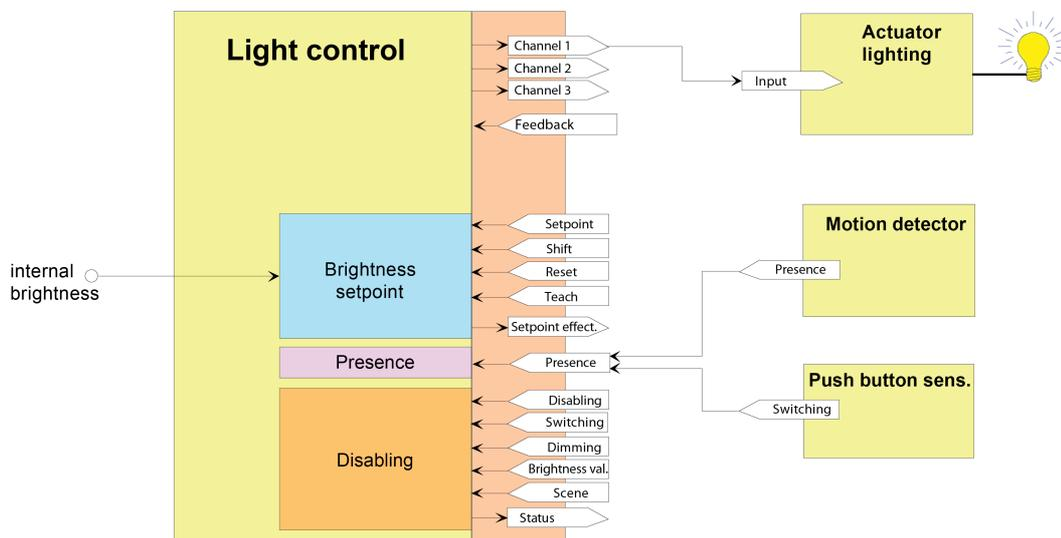
Figure 41: Application example for light control in autonomous operation
