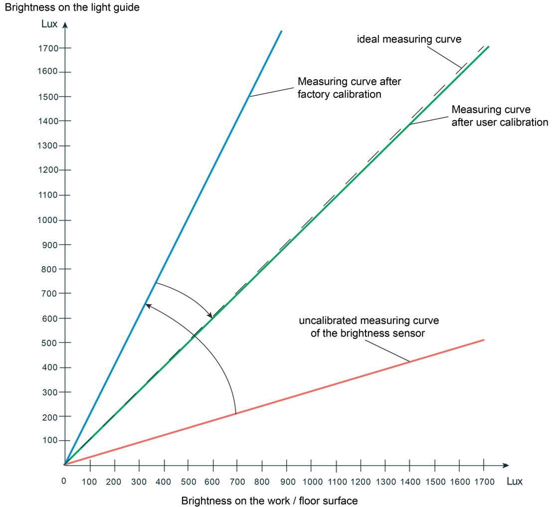
Figure 15: Correction of the determined brightness on the work / floor surface by means of user calibration
