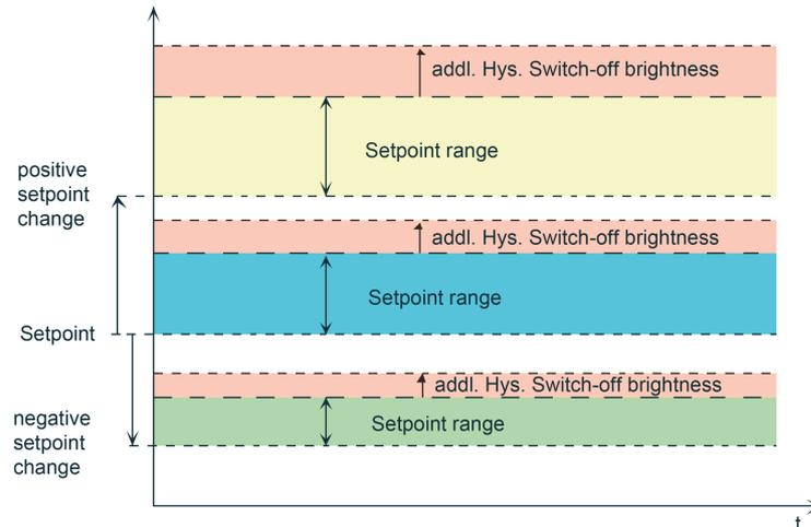
Figure 55: Dependency of the additional hysteresis for the switch-off brightness during a setpoint shift
