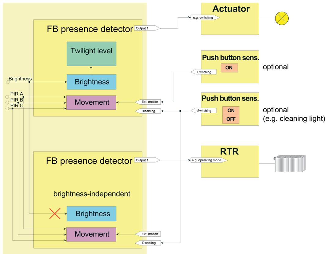
Figure 18: Application example of the application presence detector
