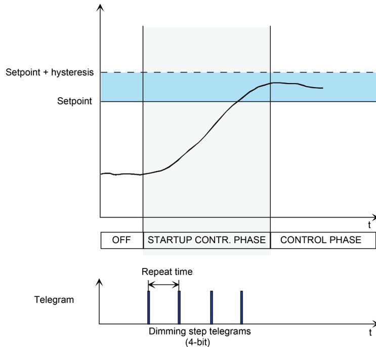
Figure 50: Startup control behaviour with relative dimming step telegrams (4-bit)
