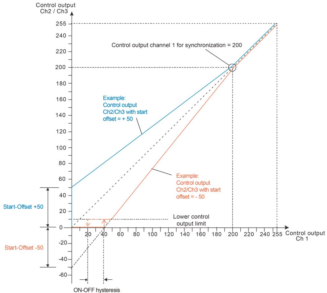
Figure 48: Control outputs of channels 2 or 3 dependent on the control output of channel 1
