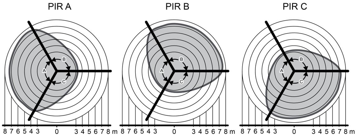
Figure 5: Detection field with PIR sectors A, B and C at an installation height of 2.50 m
