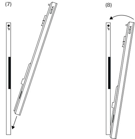
Fig. 5: Swivelling in the Display module
