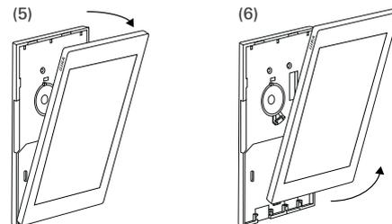
Fig.3: Removing Display module
