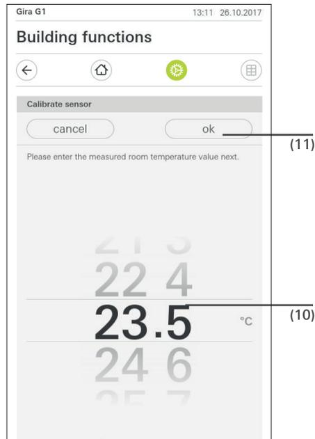
Fig. 8: [Calibrate sensor] view
