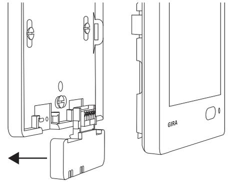
Fig. 4: Inserting temperature sensor module
