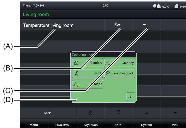
Figure 30: Example of operating and display elements of the function "Operating mode switchover KNX"
