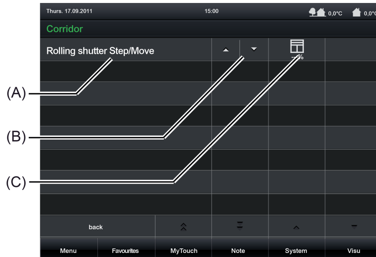
Figure 24: Example of operating and display elements of the function "Rolling shutter Step/Move"
