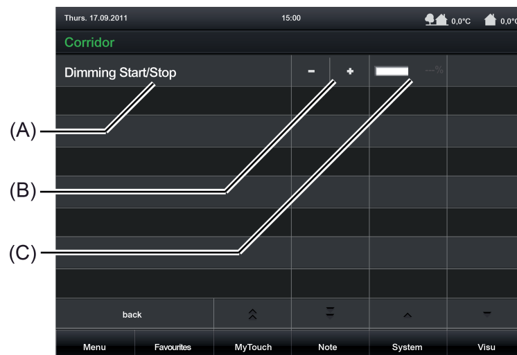
Figure 18: Example of operating and display elements of the function "Dimming (Start / Stop)"
