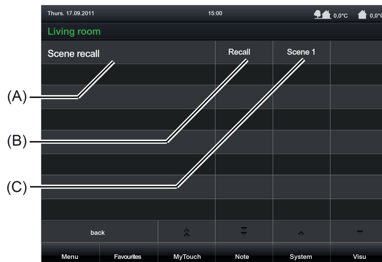
Figure 28: Example of operating and display elements of the function "Scene recall"
