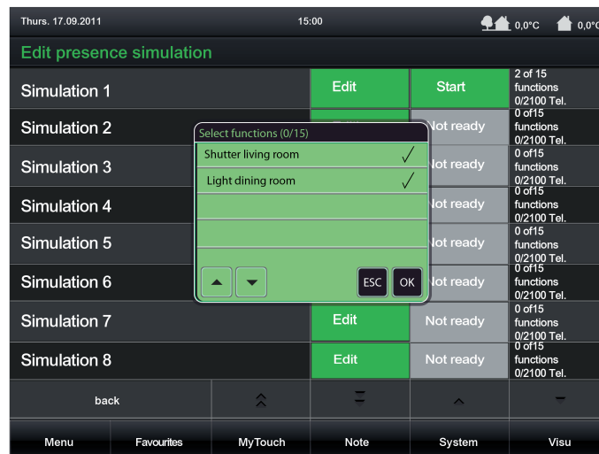
Figure 64: Example of a dialog menu for selecting functions
