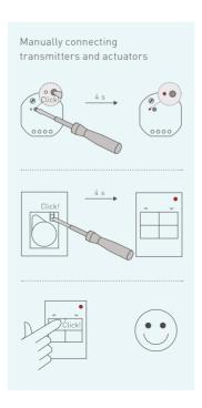
pressed. The transmitter button is now connected to the ten actuators.
