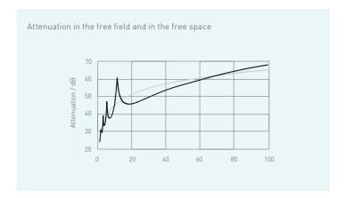
spherical shape. In the far field – at 868 MHz from approx. 2 m – the radiation power arriving at the receiver drops to the square as the distance increases. The attenuation on the transmission path is specified in decibels [dB] in technical documentation.
