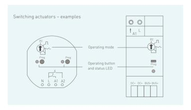
manner: A switch-on signal moves the relay permanently into the active state, while a switch-off signal moves the relay permanently into the passive state.
