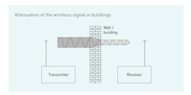
Caution is advised if a building is equipped with shielding materials to reduce "electro smog". Flush-mounted boxes with conductive coatings are hardly suitable for wireless products; special shielding plasters and gypsum cardboard protective panels into which conductive fibres have been incorporated reduce the penetrability for radio waves by up to 95%. The same applies to stud frames,
