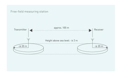
"free field", in which range measurements are performed too. The free field and the free space differ in that, in the free field, some of the radio waves are reflected on the ground and overlap with the directly radiated wave.
