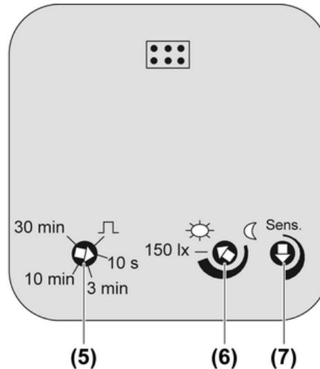
Figure 2: Adjusters on the rear
