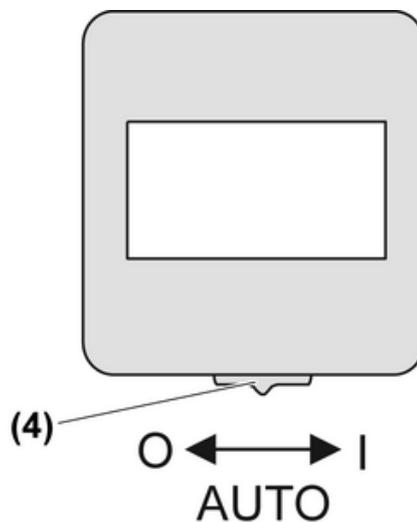
Figure 4: Operating mode switch
