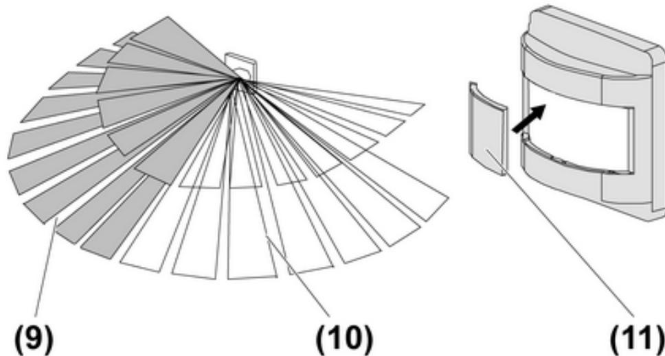
Figure 10: Using a cover plate
