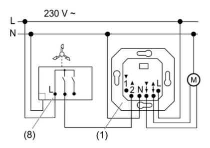
Figure 5: Connection example of wind sensor
