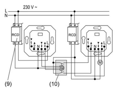
Figure 4: Connection example of two RCD circuits
