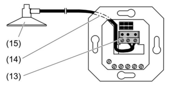
Figure 8: Surface-mounted routing of the sensor cable
