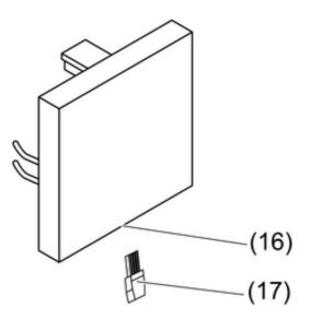
Figure 9: Sun sensor on the cover
