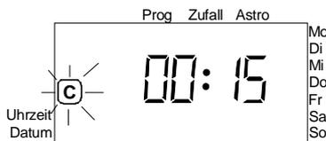
By shortly tipping (1.5 sec. max.) the **ON** key, you can start the timer function. This turns on the consumer. The display counts down.
