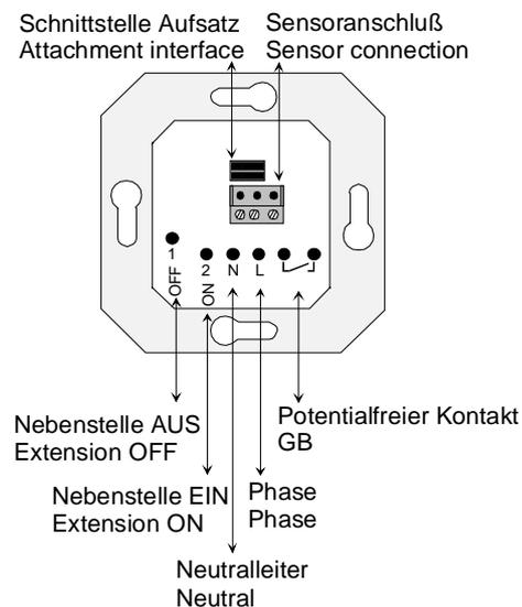
Via two separate extension inputs, the consumer can be switched by a mechanical push-button (two-key principle, 2x n. o. contacts).
