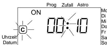
When the counter reads '0' the light is turned off. The display then reads the preset time (factory setting is 15 min.).
