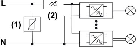
Figure 8: Connection example, surge protection module
