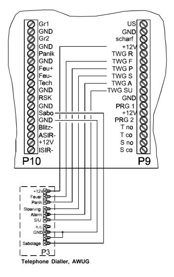
Fig. 8: AWUG Telephone Dialler Connection
