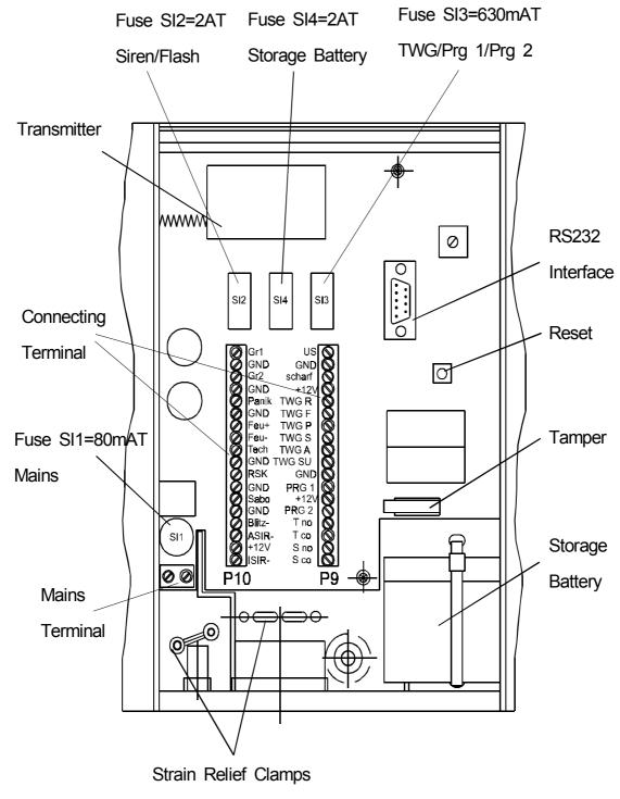
Fig. 9: Radio Alarm Center Terminal Board
