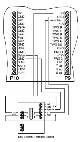
Fig. 4: Key-Operated Switch Connection to the Radio Alarm Center
