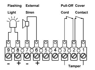
Fig. 38: External Flashing-Light Siren Terminal Assignment
