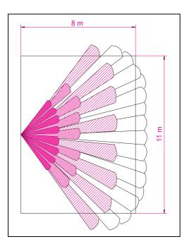
Fig. 17: Monitoring Range Vs. Installation Height
