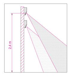
Fig. 16: Monitoring Range Top View
