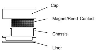
Fig. 24: Magnetic Contact Arrangement
