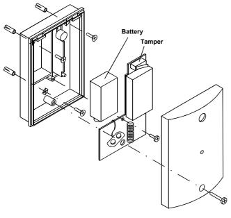
Fig. 18: Radio Glass Breakage Detector
