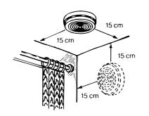
Fig. 27: Radio Smoke Detector Place of Installation
