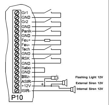
Fig. 2: P10 Connection Terminal Assignment
