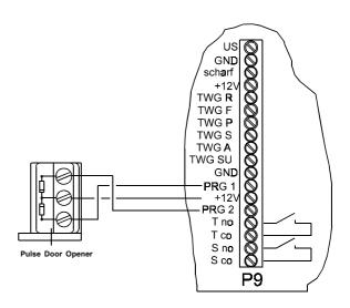
Fig 5: Pulse Door Opener Connection with the Radio Alarm Center
