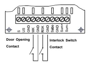
Fig. 12: Connection of Magnetic and Interlock Switch Contacts
