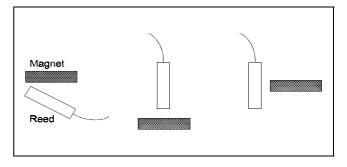
Fig. 23: Wrong Mounting of the Magnetic Contacts
