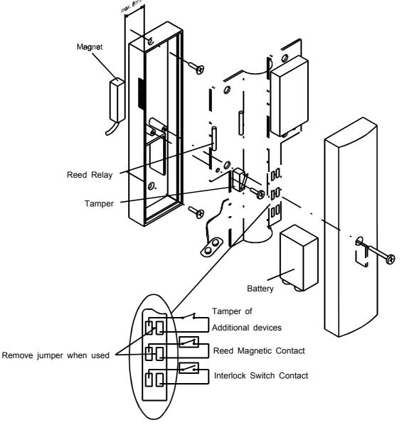
Fig. 20: Radio Magnetic Contact
