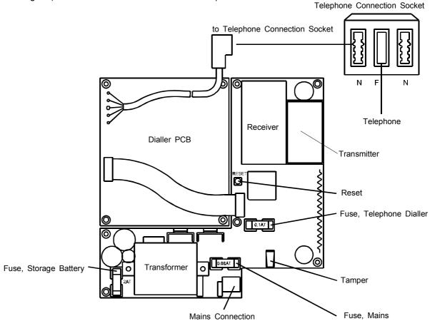
Fig. 35: AWUG Radio Telephone Dialler Connection Diagram
