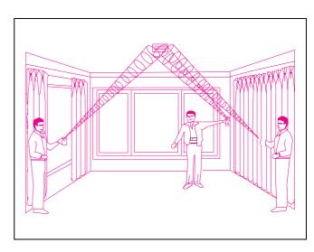
Fig. 19: Acoustic Radio Glass Breakage Detector Function Test
