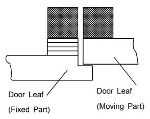
Fig. 25: Magnetic Contact Door/Window Mounting Example
