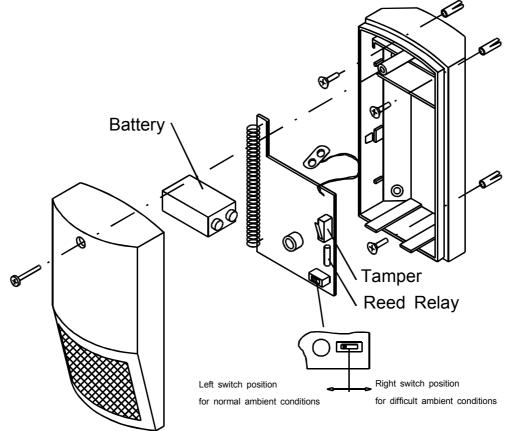
Fig. 14: Radio Movement Detector
