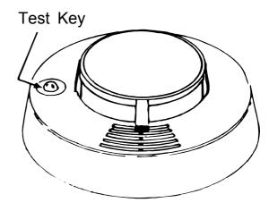
Fig. 29: Radio Smoke Detector
