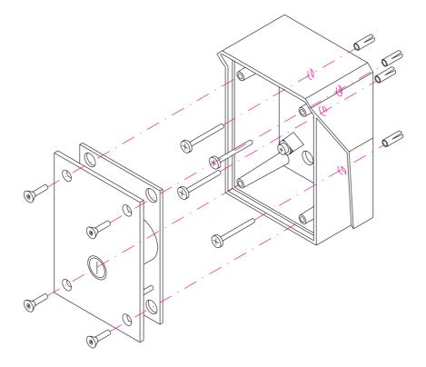
Fig. 42: Key-Operated Switch
