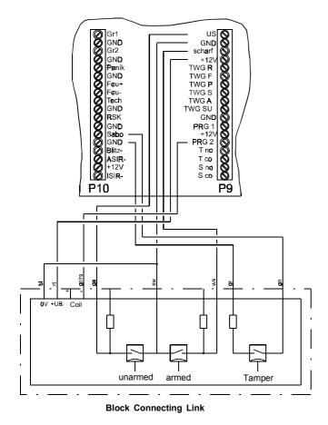
Fig 7: Example for Connecting a Block Connecting Link to the Radio Alarm Central Unit
