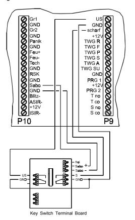
Fig. 43: Key-Operated Switch Connection to the Radio Alarm Center
