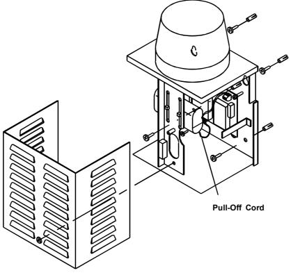
Fig. 36: Radio External Flashing-Light Siren
