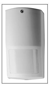
Due to specific optics (a so-called Fresnel lens) fan-shaped observation of the space within a detection range of  $8 \times 11 \text{ m}$ (90°) is possible for an installation height of 2.4 m.
