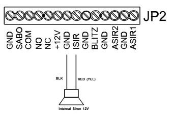
Fig. 41: Connection of the Internal Siren to the RadioSubcenter
