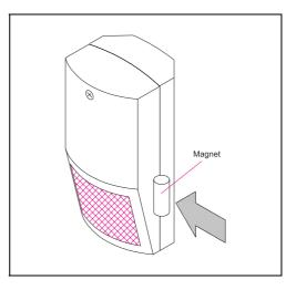
Fig. 15: Performing the Walking and Transmitting Test
