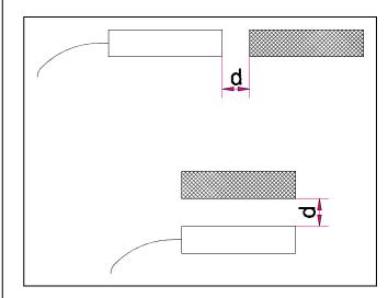
Fig. 22: Correct Fitting Position of the Magnetic Contacts
