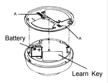
Fig. 28: Radio Smoke Detector
