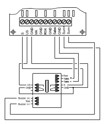
Fig. 44: Key-Operated Switch Connection to the Radio Door Module
