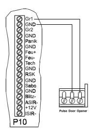
Fig 6: Opening Contact Connection
