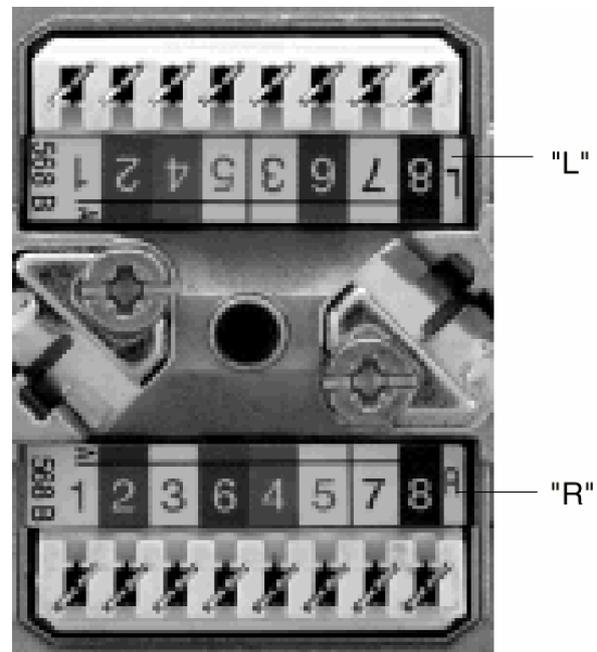
"L" = Terminal block for left connection socket (when viewed from front while installed).
