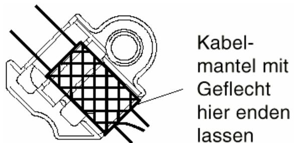
Push prepared cable end forward up to edge of cable clamp when laying into the box so that braiding lies under shield tap.
