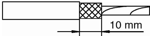
Cut off shield and plastic foil so that approx. 10 mm extends from plastic sheath
