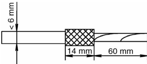
With thinner cables (under 6 mm dia.), braiding is pushed back over sheath and shortened to 14 mm
