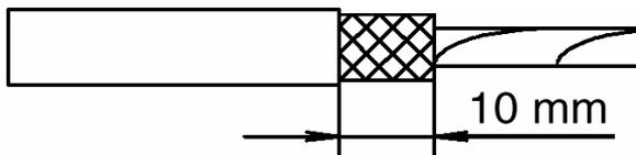
Push back braided shield and cut off all round so that approx. 10 mm extends from plastic sheath
