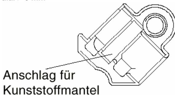
Shorten and prepare cable. **For plastered-in cables, ensure a minimum length of approx. 140 mm up to wall!**
