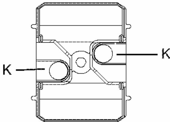
For cables with a diameter over 10 mm, we recommend opening the cable entries (K) in the cover at the marked points with a pair of diagonal cutters after laying on the wires
